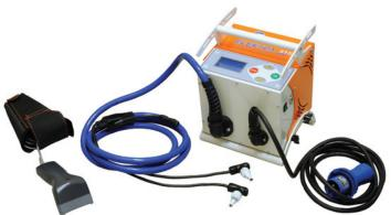
The electrofusion process involves the use of moulded socket fittings containing an electric heating coil. The pipe ends are inserted into the sockets and clamped. An electrical current is then passed through the coil for a pre-set time. Heating of the surrounding plastic and heat transfer to the pipe wall then takes place. This process is commonly used where space is limited and/or lateral pipe movement is not possible.
