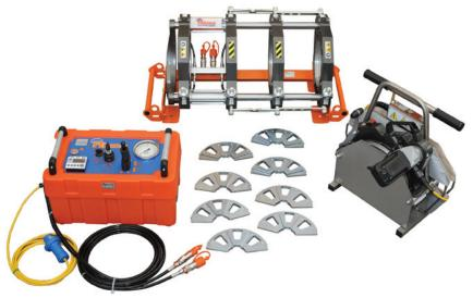
This technique is generally used for pipe and fittings ranging from 6" and larger. The process involves the joining of plain-end pipe with plain-end fittings. The pipe and fittings are heated while being pressed against a "heated plate" for a specified period of time. The heat is absorbed into the pipe and fitting, allowing them to weld together, and then cooled. Welding and cooling time is determined by the pipe diameter and wall thickness.
